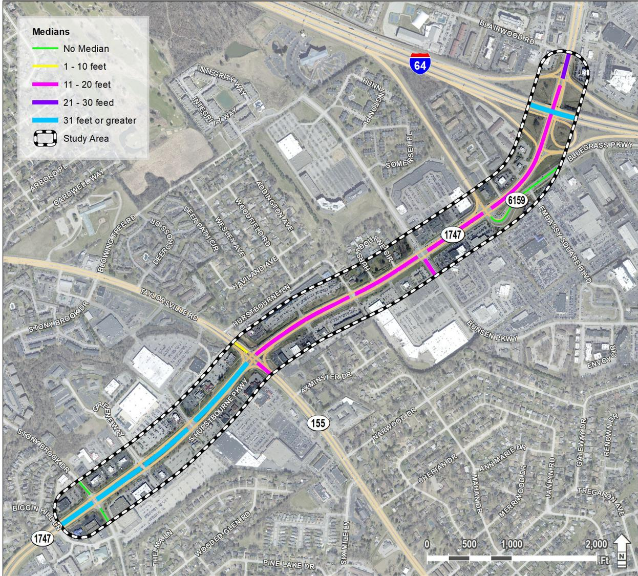
Figure 7: Median Widths along Study Corridor
