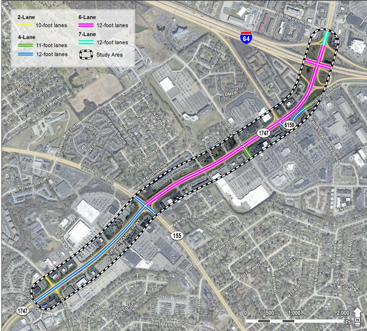
Figure 4: Lane Widths along Study Corridor
