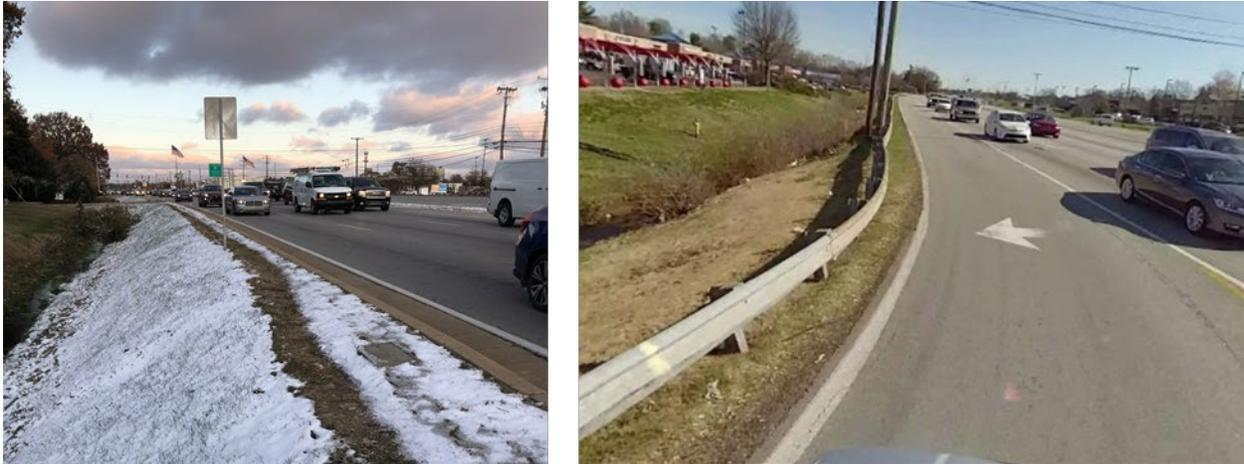
**Figure 12: Roadside Pedestrian Path in Lieu of Sidewalk**
