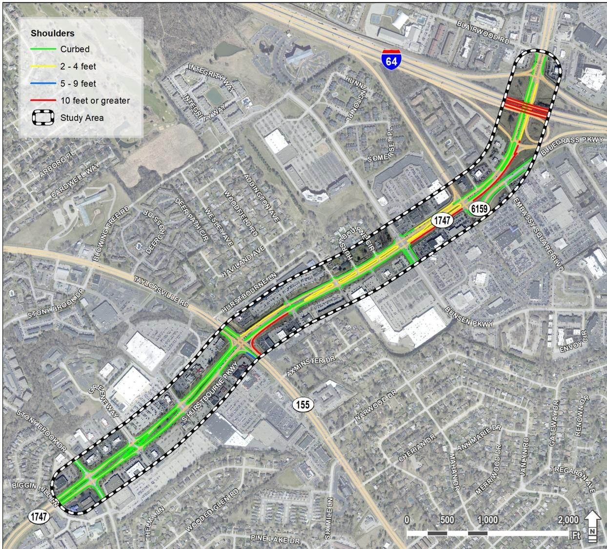
**Figure 5: Shoulder Widths along Study Corridor**
